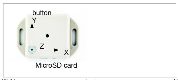
The positive axis orientations are shown in the diagram above.
